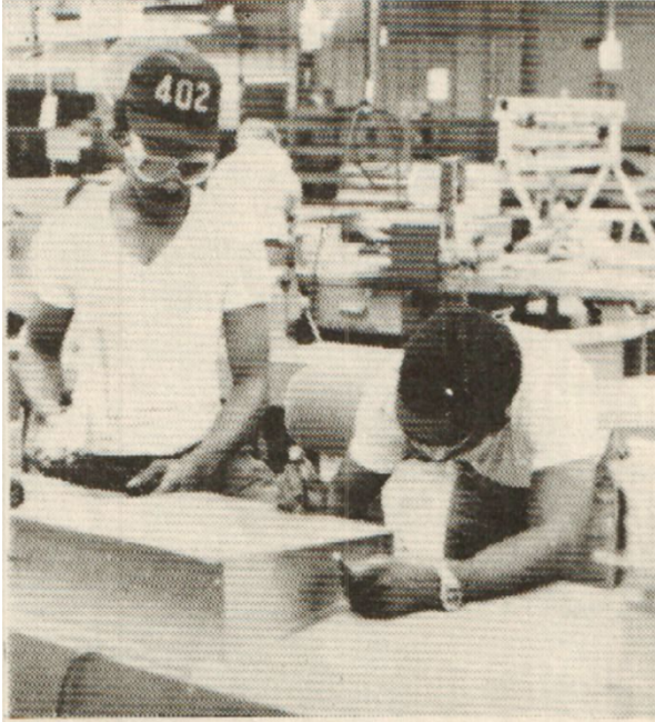
Sgt James Folson, Left watches as Sgt Issac Sampson checks his rivet work for proper height.
